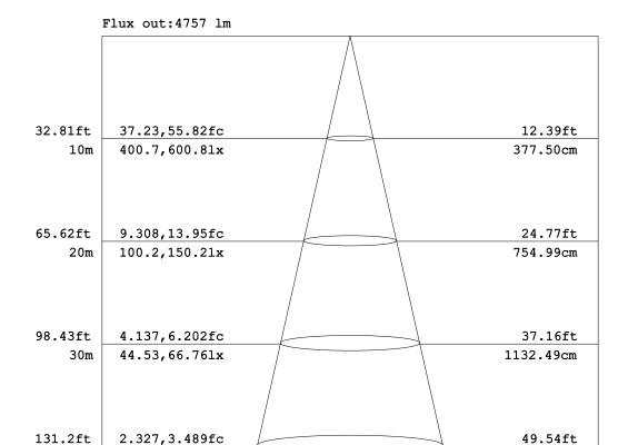
Note: The Curves indicate the illuminated area and the average illumination when the luminaire is at different distance.
