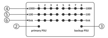
The XES-8G has three status LEDs for each of the network ports plus a status LED for either of the power supplies. The LED for the primary PSU (2) and the LED for the backup PSU indicate whether the respective PSU is powered from the mains and functioning.
