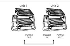
NOTE: when not using the Power output connectors, you must seal the cable ends with the supplied caps.
