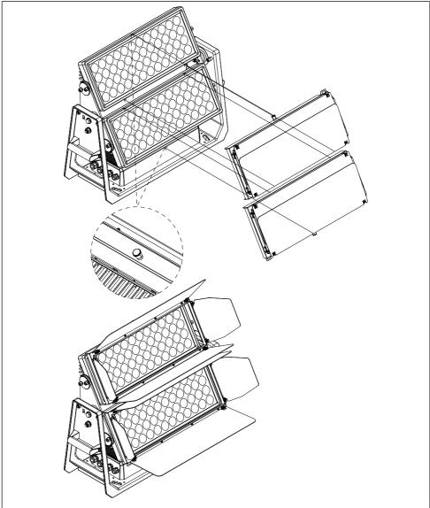
Insert the three to positioning and the spring pin on the hardware into the holes provided on the top and down side edge of the product.
