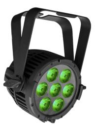
**LumiPar** 7IP is a compact and flexible IP LED PAR made for small concerts and theatres, and to perform as architectural accent luminaire for outdoor events. The housing in die-cast aluminium is designed to feature both as a robust workhorse and totally fan-free being totally silent during its operation.
