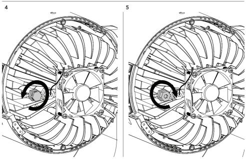
Remove the gore valve on the rear connection heatsilk module (4) and insert the hex socket cap head included in the IPTESTBOX box (5).
