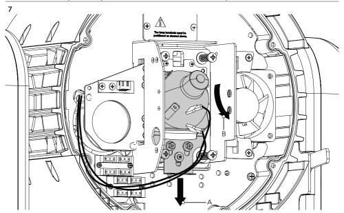
Push the metal locking plate down (A) and remove the lamp (B).
