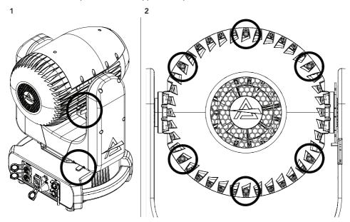
Before removing rear cover, place the head in a right-angle horizontal position and engage both the PAN and TILT locks for added stability while replacing the lamp (1). See the "PAN AND TILT LOCK" paragrap. Then remove the six market screws to remove rear cover (2).
