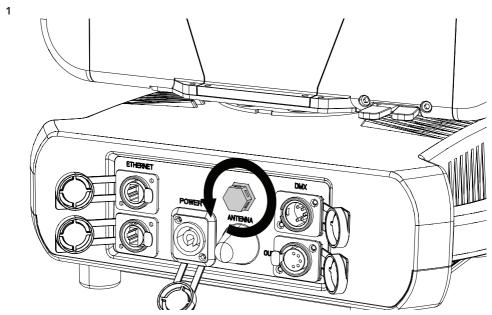
Remove the gore valve from the connections panel.
