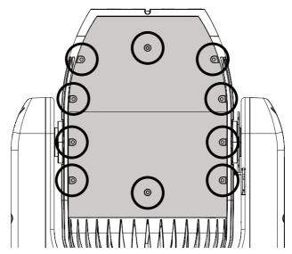
Before removing rear cover, place the head in a horizontal position and engage both the PAN and TILT locks for added stability. See the "PAN AND TILT LOCK" paragrap.
