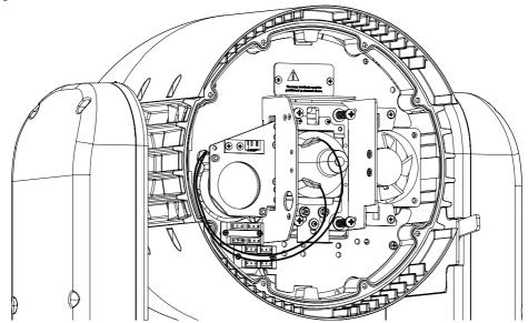
Slow remove the spade receptacle-terminals connected to the lamp.
