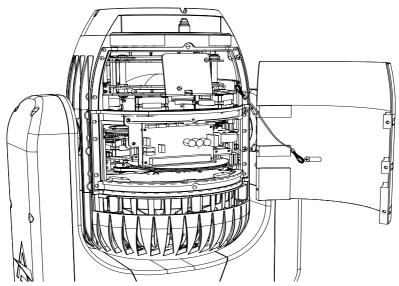
Unclip the heatsink module safety cable.
