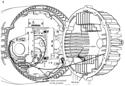
Unclip the heatsink module safety cable. Slow remove the cable connected to the module and remove the heatsink module.
