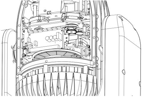
Use a soft cloth dampened with any detergent liquid for cleaning glass to remove the dirt from the reflectors, from the lenses and filters.
